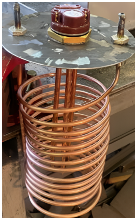
Figure 4. A coil heat exchanger is used to heat carbon dioxide.
